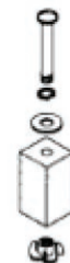
Figure 6 Slotted Head Boat Lock Washer Mounting Strap Mounting Block Tree-Nut Imbedded In Block
